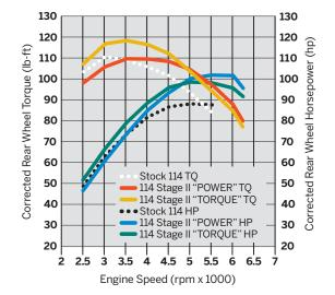
\*\* FLHXSE 114 Stage II "POWER" with Ventilator A/C & Street Cannon Mufflers \*\* FLHXSE 114 Stage II "TORQUE" with Heavy Breather A/C & Street Cannon Mufflers
