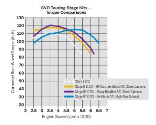
DYNAMOMETER (DYNO) PERFORMANCE TESTING: Declared performance values in this catalog represent SAE J-1349 transient peak power output. Dynamometer settings, motorcycle condition, variation, climate and other factors can affect performance output and results can vary from the performance values declared by Harley-Davidson.
