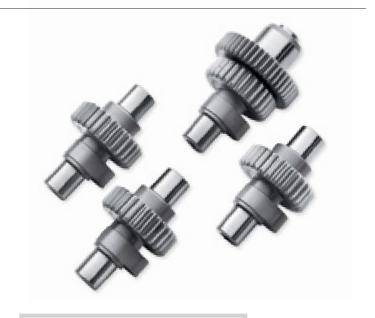
Stage II upgrade requires minor engine disassembly to replace the cam. Special tools and ECM tuning are required.
